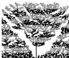
Fig. 8.5 Ballistic growth from an interface initially containing a point irregularity. The initial interface consists of 100 sites and a column of size 35. The colour was changed after each 800 atoms had been deposited
